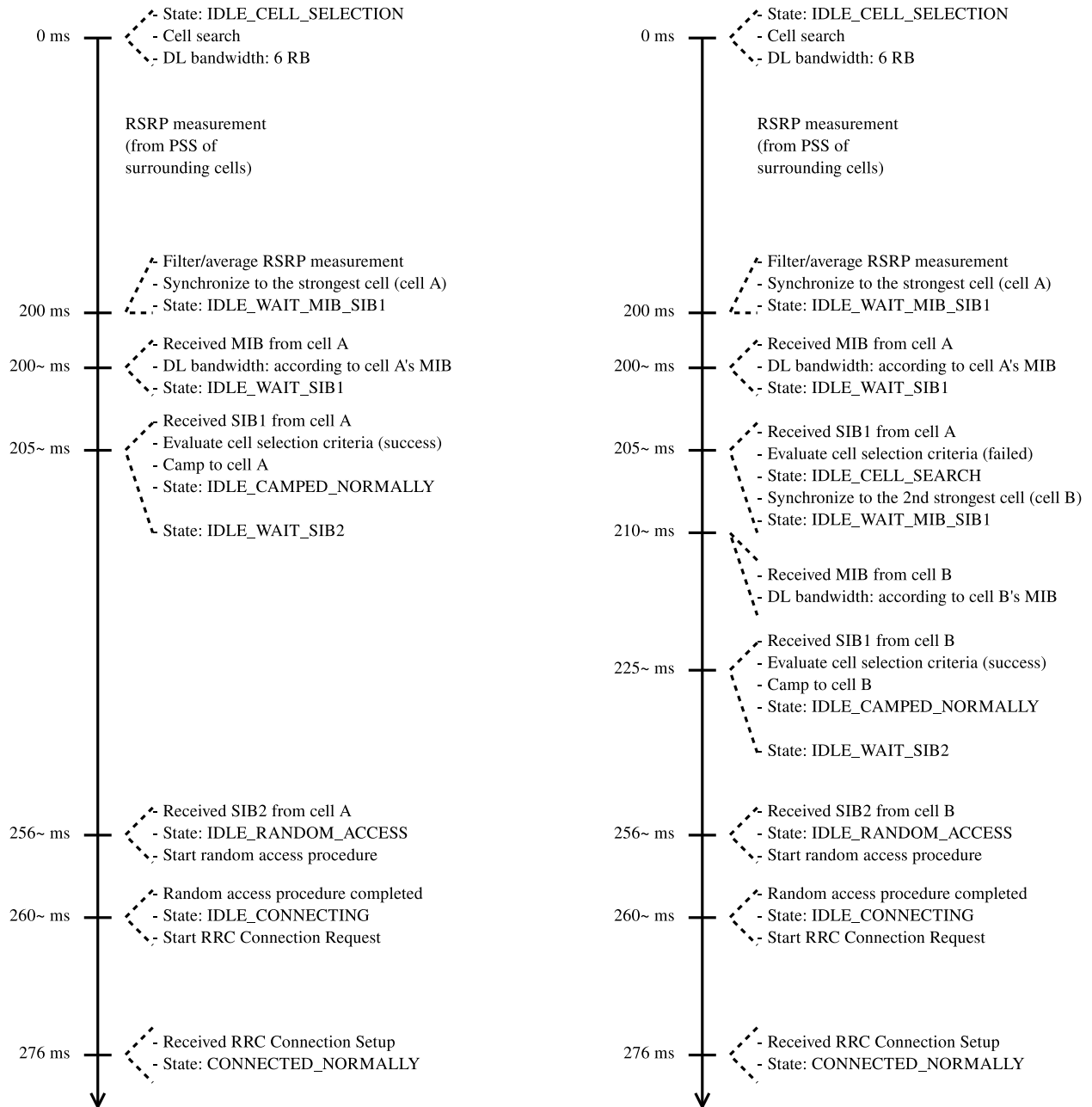
Fig. 32: Sample runs of initial cell selection in UE and timing of related events
