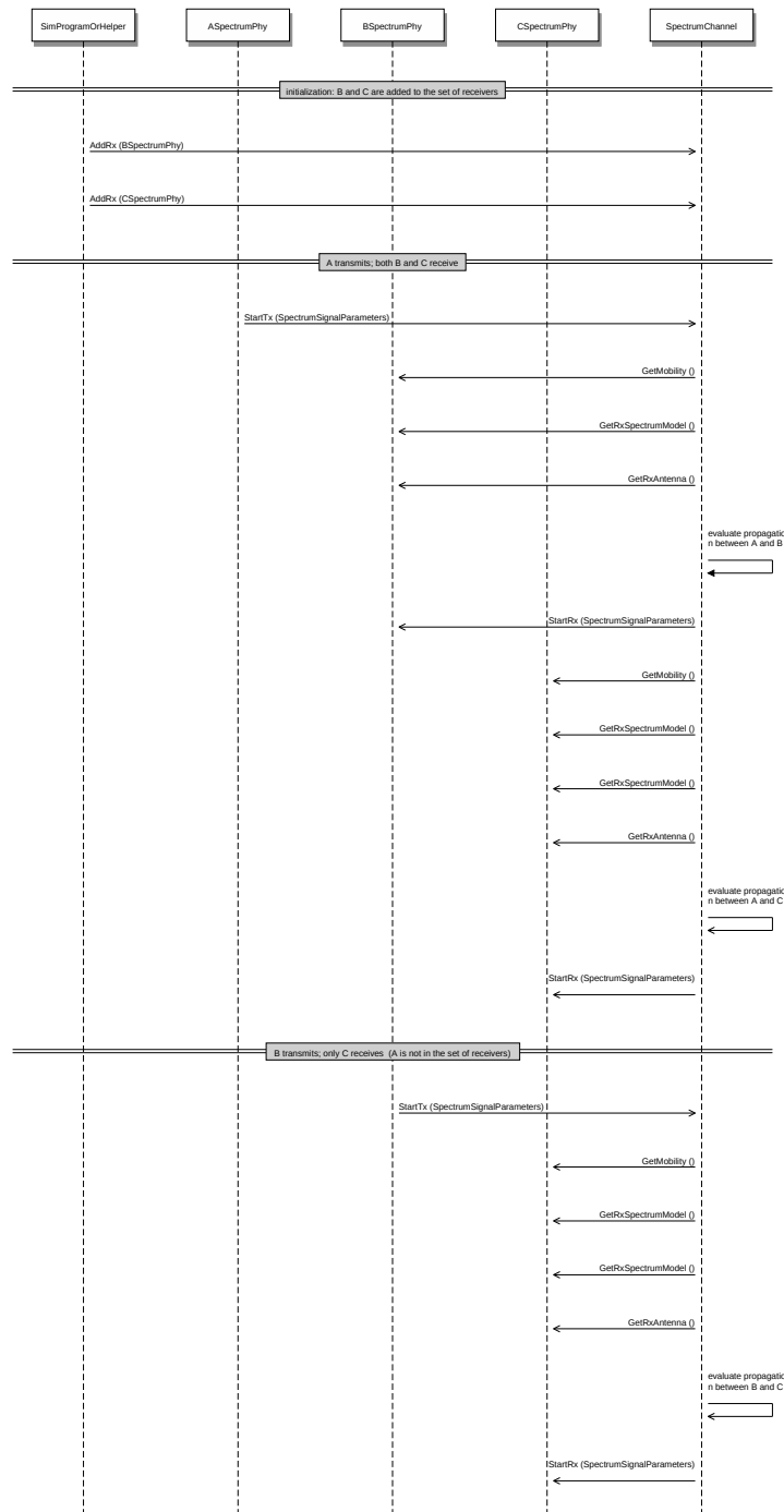
Fig. 2: Sequence diagram showing the interaction between SpectrumPhy and SpectrumChannel
