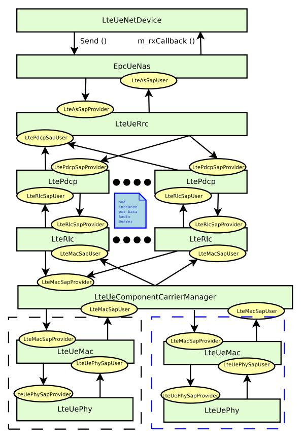
Fig. 67: UE Data Plane Architecture
