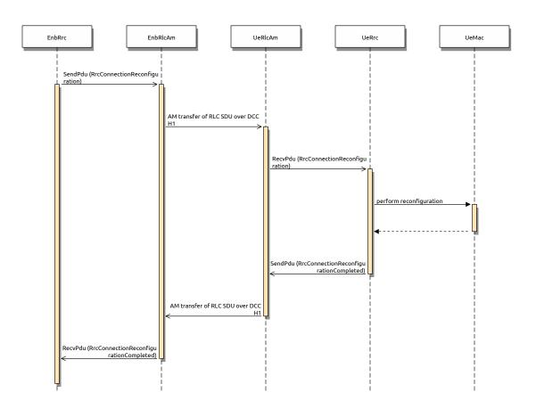
Fig. 40: Sequence diagram of the RRC Connection Reconfiguration procedure
