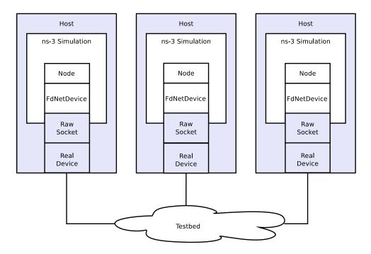
Fig. 1: Example Implementation of Testbed Emulation.
