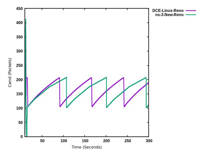
Fig. 8: DCE Linux Reno vs. ns-3 NewReno
