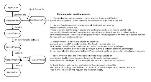
Fig. 1: Send path of a packet.
