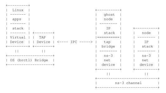
In this case, a computer running Linux applications, protocols, etc., is connected to a ns-3 simulated network in such a way as to make it appear to the Linux host that the TAP device is a real network device participating in the Linux bridge.
