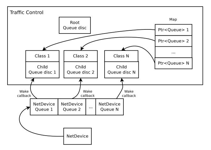
Fig. 2: Setup of a multi-queue aware queue disc
