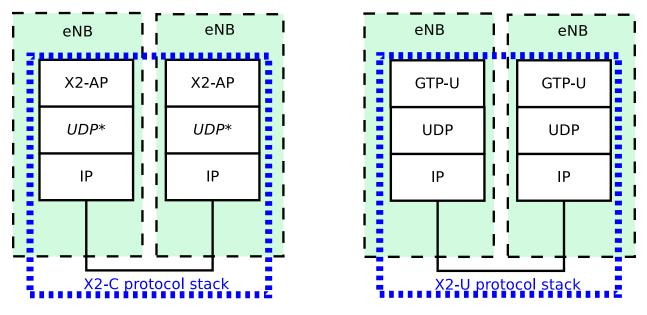
Fig. 47: X2 interface protocol stacks
