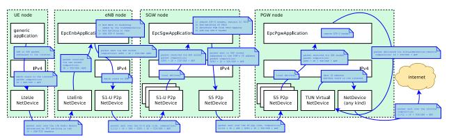
Fig. 44: Data flow in the uplink between the UE and the internet
