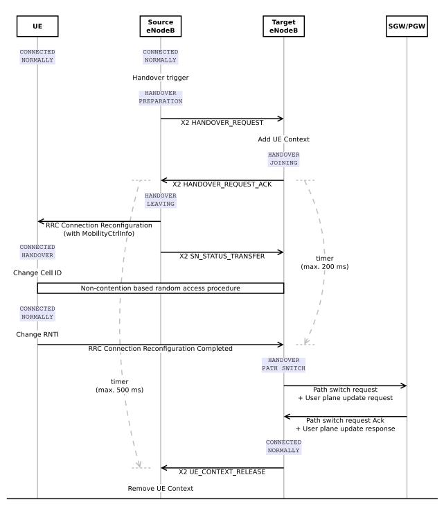
Fig. 45: Sequence diagram of the X2-based handover
