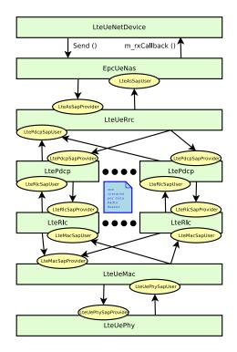
Fig. 2: LTE radio protocol stack architecture for the UE on the data plane
