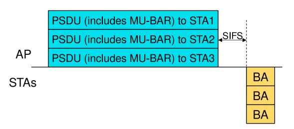
Fig. 10: Acknowledgment of DL MU frames via aggregated MU-BAR Trigger Frames
