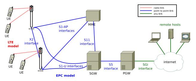
Fig. 1: Overview of the LTE-EPC simulation model
