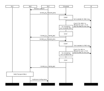
Fig. 49: Sequence diagram of Scheduling with FR algorithm
