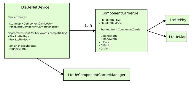
Fig. 62: Changes in LteUeNetDevice to support CA
