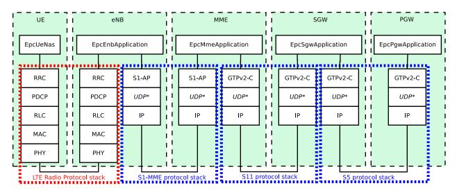
Fig. 9: LTE-EPC control plane protocol stack
