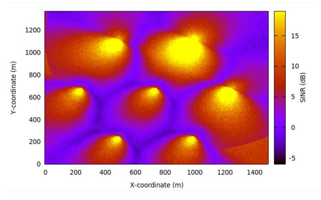
Fig. 80: REM for RB 20 obtained from lena-dual-stripe simulation with Hard FR algorithm enabled
