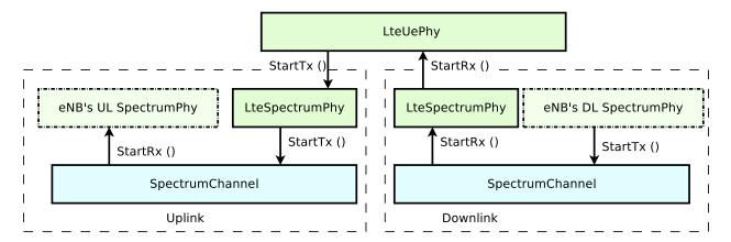
Fig. 4: PHY and channel model architecture for the UE
