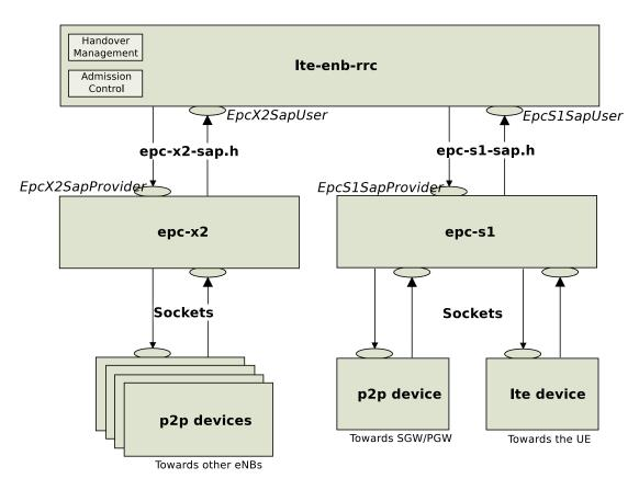
Fig. 46: Implementation Model of X2 entity and SAPs
