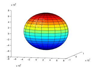
Fig. 5: Plot from MATLAB implementation of CreateRegionalTvTransmitters method in TvSpectrumTransmitterHelper. Shows 100 random points on Earth's surface (with altitude 0) corresponding to TV transmitter locations within a 2000 km radius of 35° latitude and -100° longitude.
