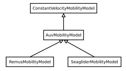
Fig. 1: AUV's mobility model classes overview
