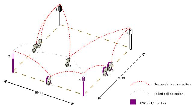
Fig. 97: Sample result of cell selection test
