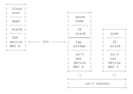
In this case, the pre-configured MAC address of the "Tap device" (MAC X) will not be the same as that of the bridged "ns-3 net device" (MAC Y) shown in the illustration above. In order to bridge to ns-3 net devices which do not support SendFrom() (especially wireless STA nodes) we impose a requirement that only one Linux device (with one unique
