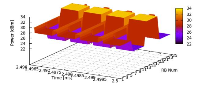
Fig. 77: Spectrum Analyzer trace obtained from lena-frequency-reuse example with Soft FFR algorithm enabled. Spectrum Analyzer was located need eNB with FrCellTypeId 2.
