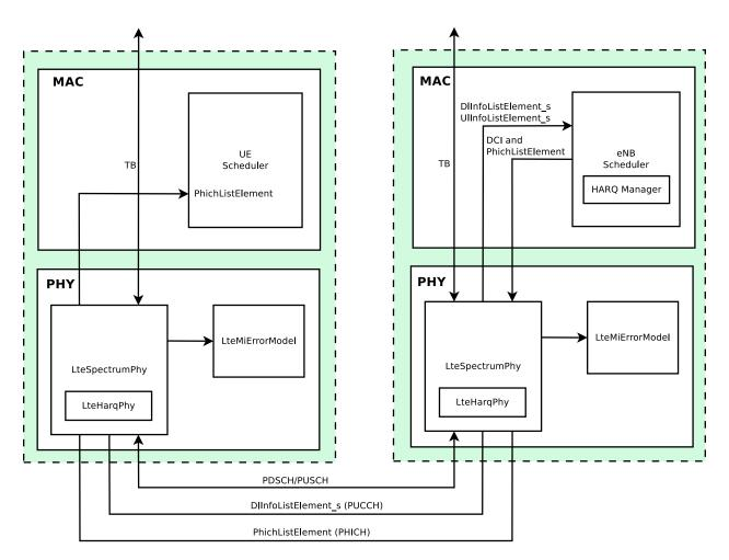
Fig. 22: Interaction between HARQ and LTE protocol stack
