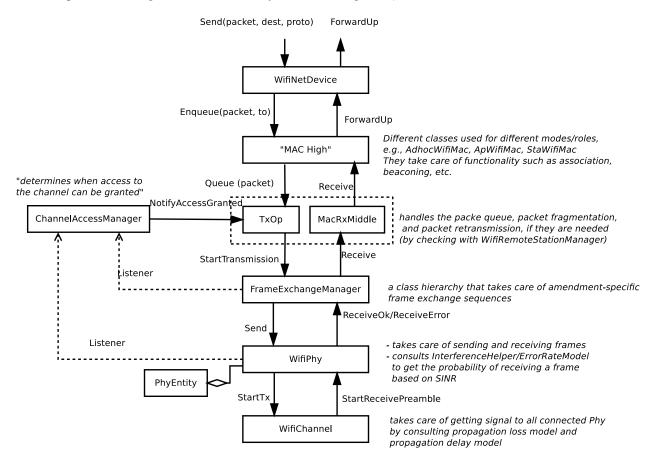
Fig. 1: WifiNetDevice architecture
