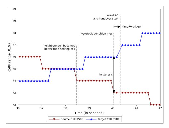
Fig. 38: Effect of hysteresis and time-to-trigger in strongest cell handover algorithm
