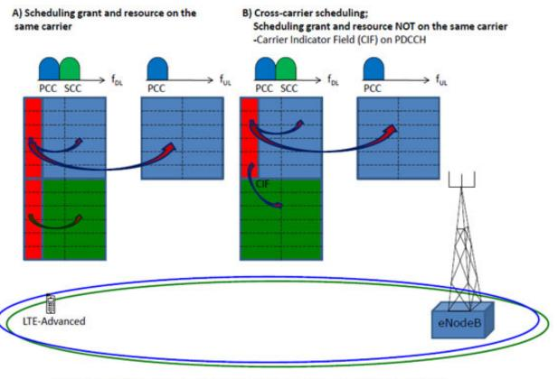
Primary Serving Cell (PSC), Primary Component Carrier (PCC), RRC connection and data Secondary Serving Cell (SSC), Secondary Component Carrier (SCC), user data
