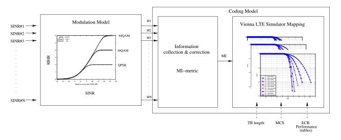
Fig. 12: MIESM computational procedure diagram
