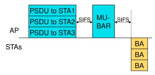
Fig. 9: Acknowledgment of DL MU frames via MU-BAR Trigger Frame sent as single-user frame
