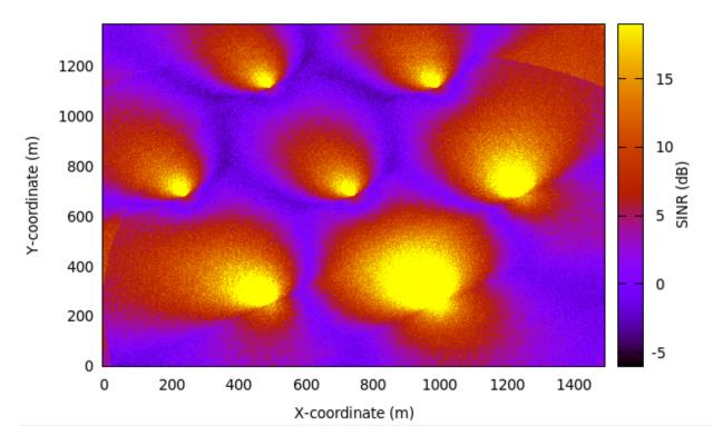
Fig. 79: REM for RB 10 obtained from lena-dual-stripe simulation with Hard FR algorithm enabled
