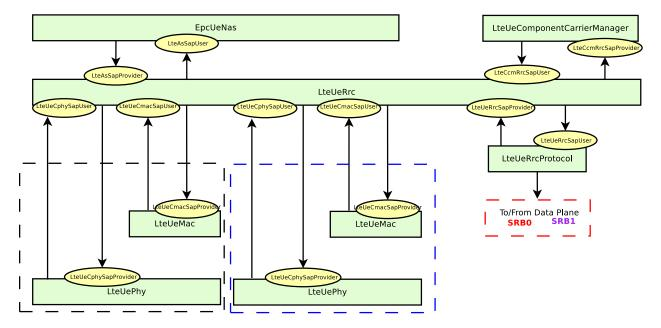
Fig. 69: UE Control Plane Architecture
