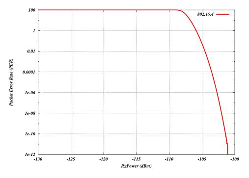
Fig. 3: Packet error rate vs. signal power
