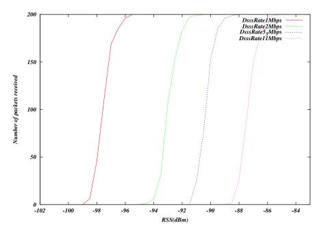
Fig. 12: Clear channel (AWGN) error model for 802.11b
