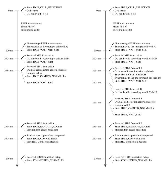
Fig. 32: Sample runs of initial cell selection in UE and timing of related events
