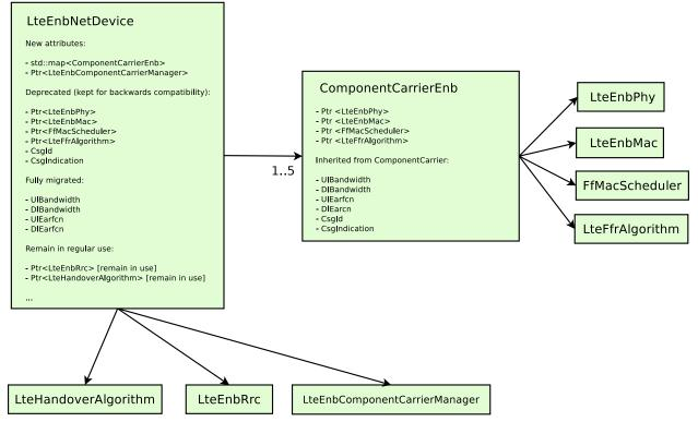
Fig. 61: Changes in LteEnbNetDevice to support CA
