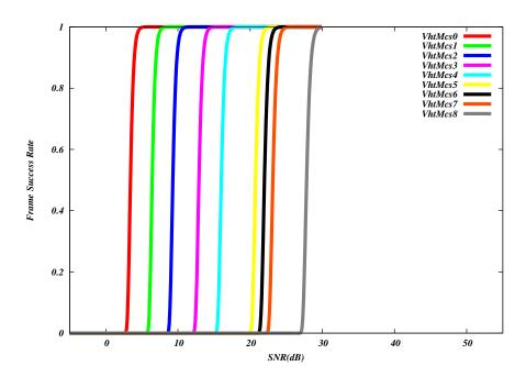
Fig. 15: Frame error rate (NIST model) for 802.11ac (VHT OFDM) Wi-Fi
