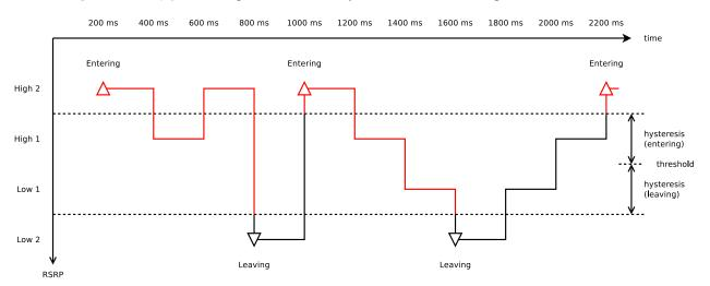
Fig. 91: Measured RSRP trace of an example Event A1 with hysteresis test case in piecewise configuration
