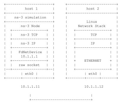
This helper replaces the functionality of the EmuNetDevice found in *ns-3* prior to ns-3.17, by bringing this type of device into the common framework of the FdNetDevice. The EmuNetDevice was deprecated in favor of this new helper.
