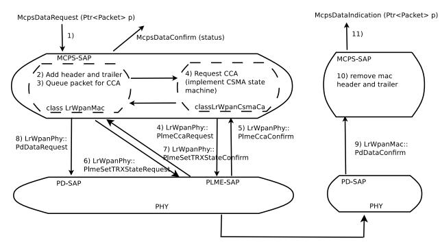
Fig. 4: Data example for simple LR-WPAN data transfer end-to-end
