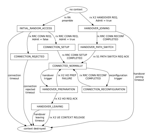
Fig. 31: ENB RRC State Machine for each UE
