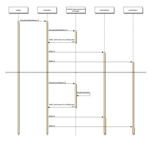
Fig. 66: Sequence Diagram of Data Radio Bearer Setup
