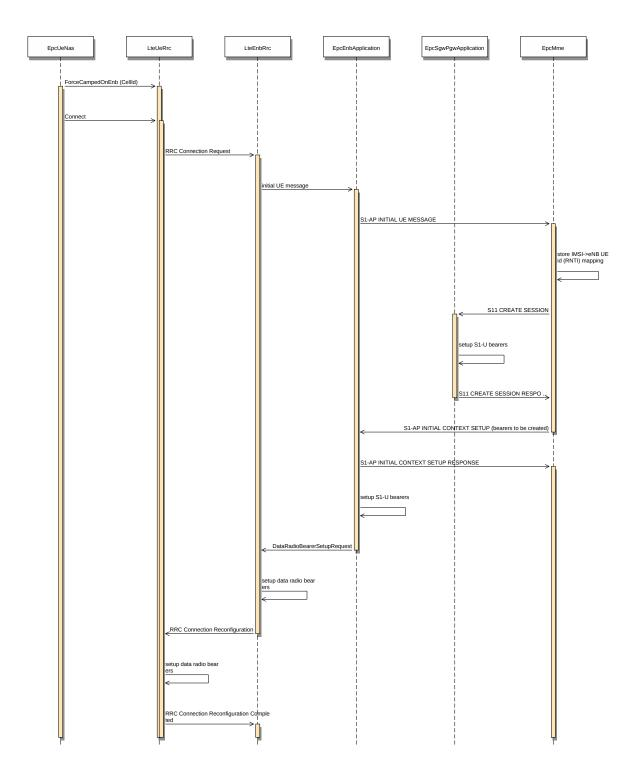
Fig. 42: Sequence diagram of the attach procedure
