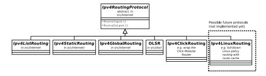
Fig. 4: Ipv4Routing specialization.
