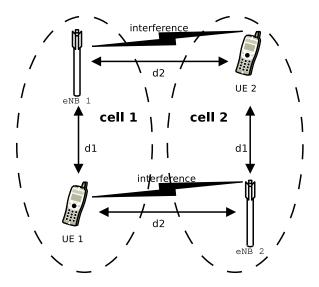
Fig. 88: Topology for the inter-cell interference test
