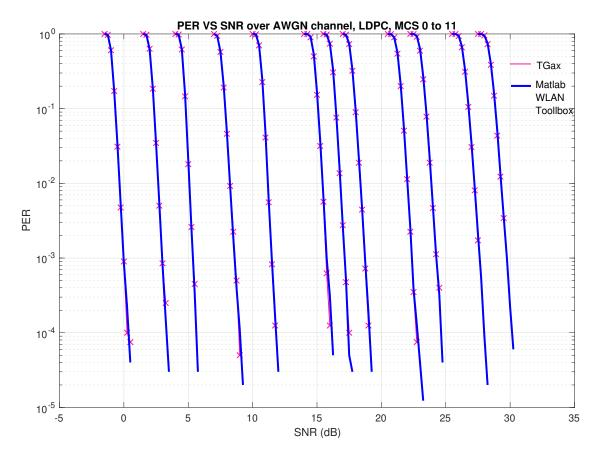
Fig. 5: Comparison of table-based OFDM Error Model with TGax results.
