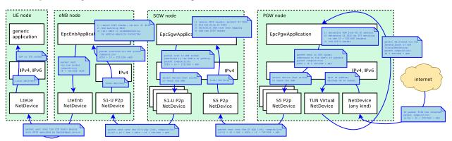
Fig. 43: Data flow in the downlink between the internet and the UE
