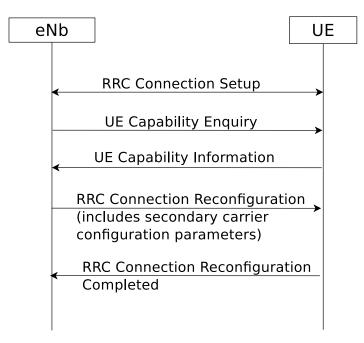
Fig. 59: A schematic overview of the secondary carrier enabling procedure
