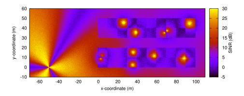
Fig. 74: REM obtained from the lena-dual-stripe example
