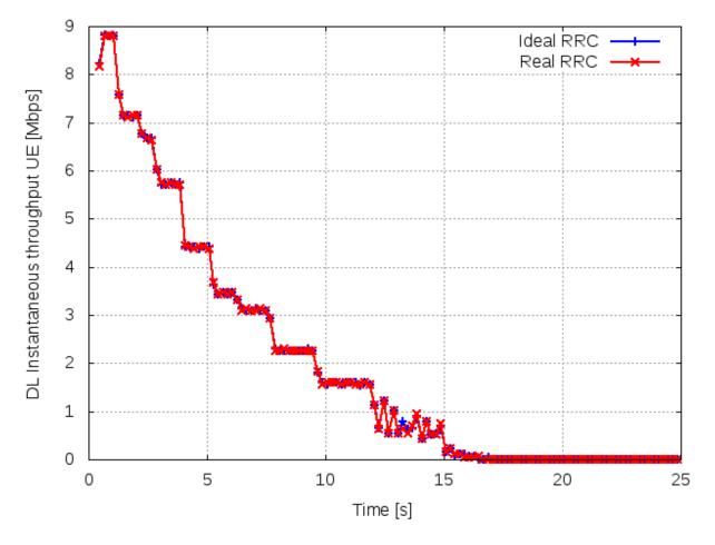
Fig. 84: Downlink instantaneous throughput of UE in scenario A
