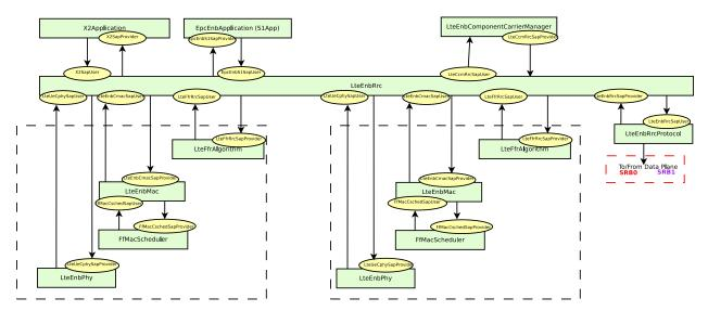
Fig. 65: eNB Control Plane Architecture
