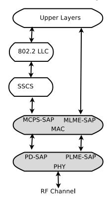
Fig. 1: Architecture and scope of lr-wpan models
