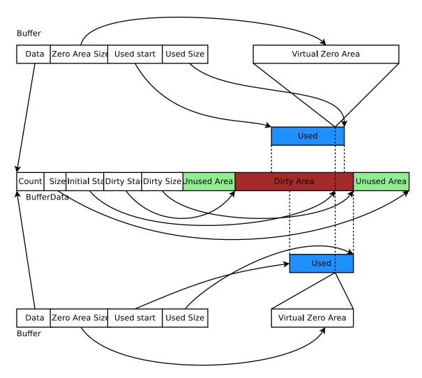
Fig. 2: Implementation overview of a packet's byte Buffer.
