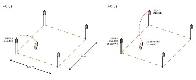
Fig. 98: lte-handover-target test scenario in a 2×2 grid
