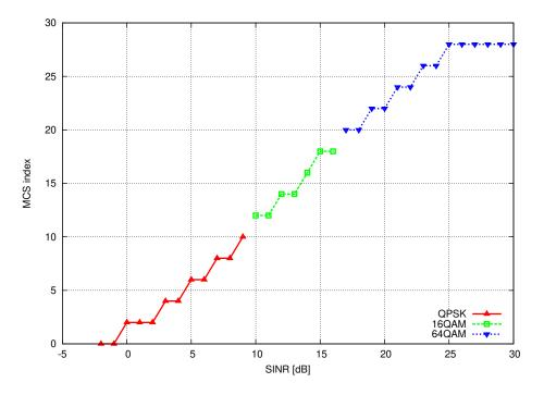
Fig. 87: Test vector for Adaptive Modulation and Coding
