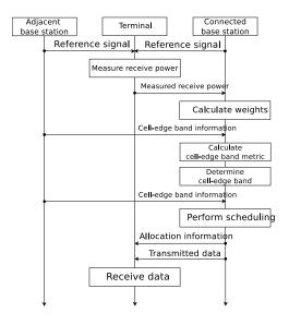
Fig. 57: Sequence diagram of Distributed Frequency Reuse Scheme
