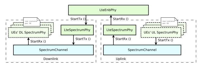
Fig. 7: PHY and channel model architecture for the eNB
