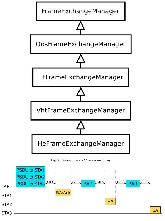
Fig. 8: Acknowledgment of DL MU frames in single-user format
