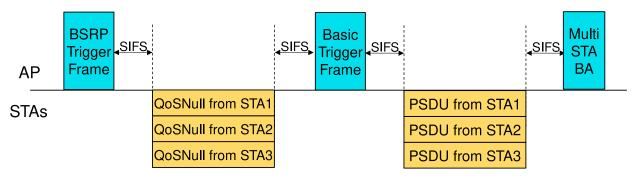
Fig. 11: Acknowledgment of DL MU frames via aggregated MU-BAR Trigger Frames
