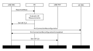
Fig. 48: Sequence diagram of Downlink Power Control
