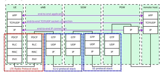
Fig. 8: LTE-EPC data plane protocol stack
