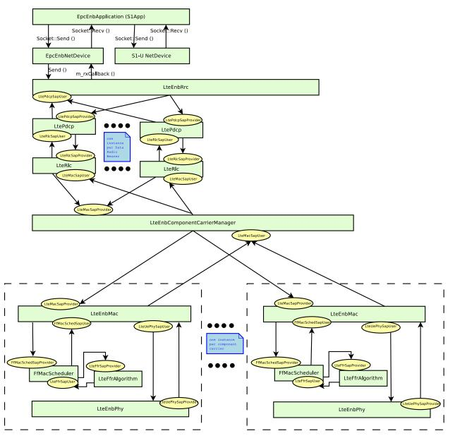
behavior, when a new logical channel is activated, the logical channel configurations is propagated to each MAC layer object in "as is" fashion.
