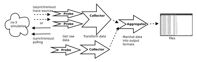
Fig. 2: Data Collection Framework aggregation
