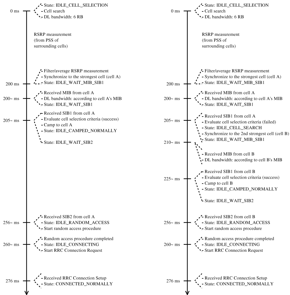
Figure 20.32: Sample runs of initial cell selection in UE and timing of related events
