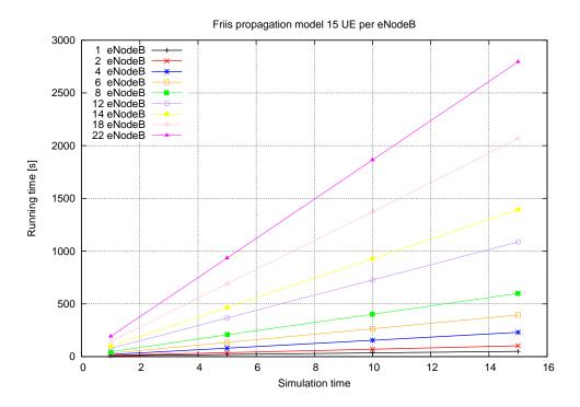
Figure 20.82: Simulation time
