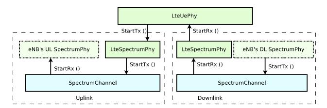
Figure 20.4: PHY and channel model architecture for the UE
