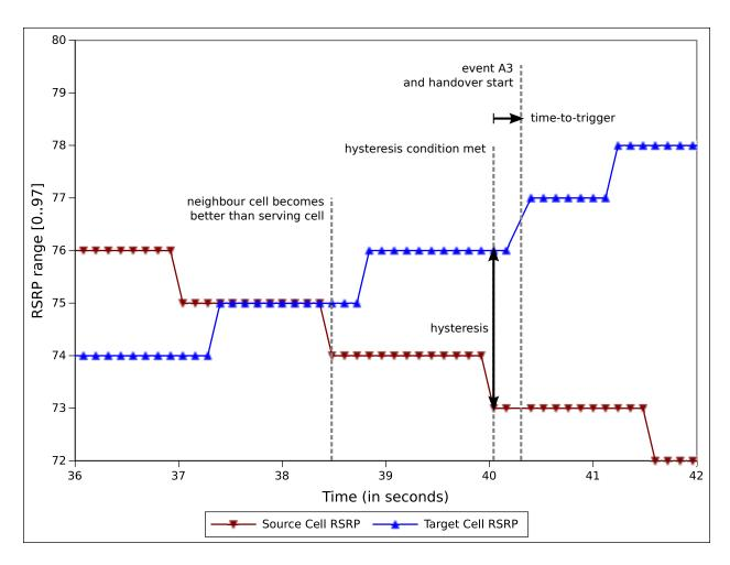
Figure 20.35: Effect of hysteresis and time-to-trigger in strongest cell handover algorithm
