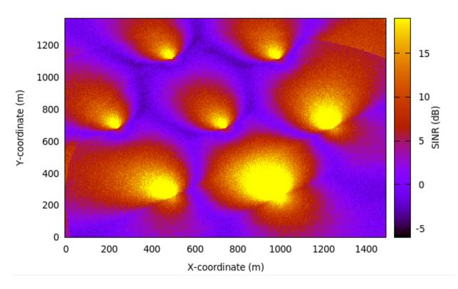
Figure 20.64: REM for RB 10 obtained from lena-dual-stripe simulation with Hard FR algorithm enabled
