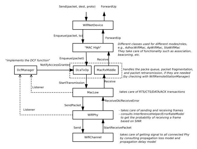
Figure 36.1: WifiNetDevice architecture.
