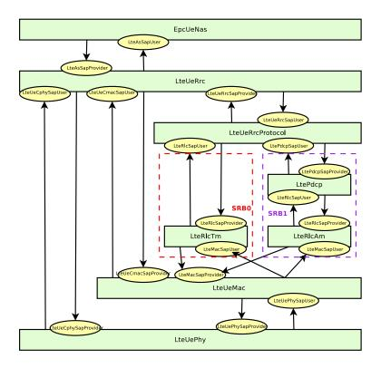
Figure 20.3: LTE radio protocol stack architecture for the UE on the control plane
