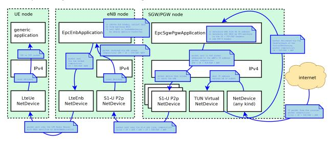
Figure 20.40: Data flow in the downlink between the internet and the UE
