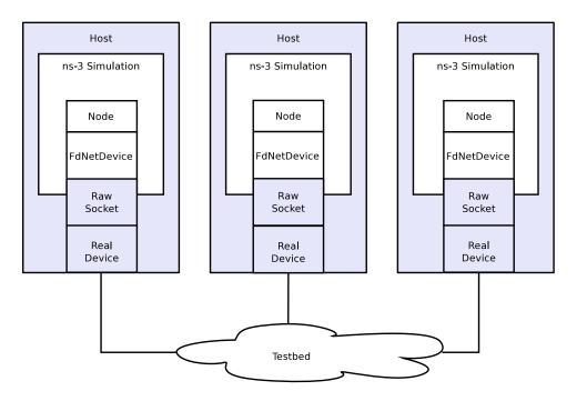
Figure 14.1: Example Implementation of Testbed Emulation.
