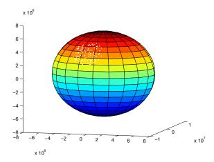
Figure 29.5: Plot from MATLAB implementation of CreateRegionalTvTransmitters method in TvSpectrumTransmitterHelper. Shows 100 random points on Earth's surface (with altitude 0) corresponding to TV transmitter locations within a 2000 km radius of 35° latitude and -100° longitude.
