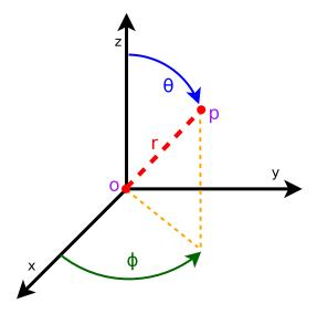
Figure 3.1: Coordinate system of the AntennaModel
