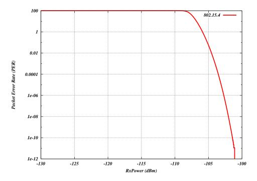
Figure 19.3: Packet error rate vs. signal power
