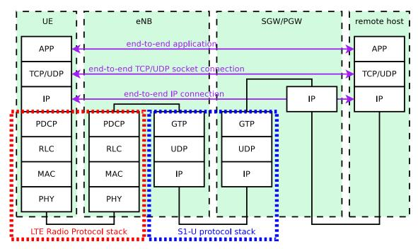
Figure 20.8: LTE-EPC data plane protocol stack
