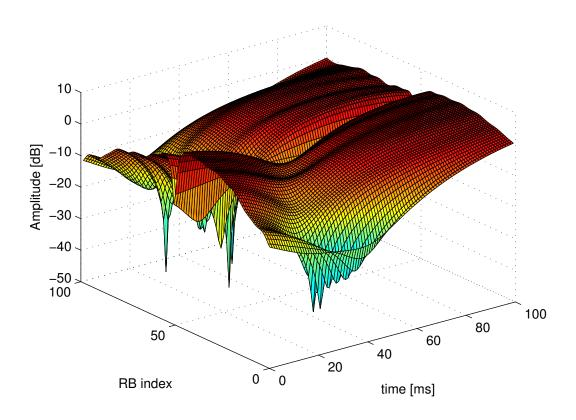
Figure 20.56: Excerpt of the fading trace included in the simulator for a pedestrian scenario (speed of 3 kmph).
