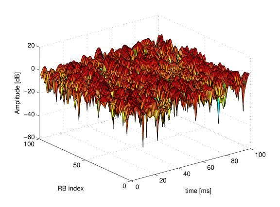
Figure 20.57: Excerpt of the fading trace included in the simulator for a vehicular scenario (speed of 60 kmph).
