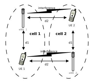
Figure 20.67: Topology for the inter-cell interference test
