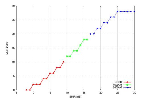
Figure 20.66: Test vector for Adaptive Modulation and Coding
