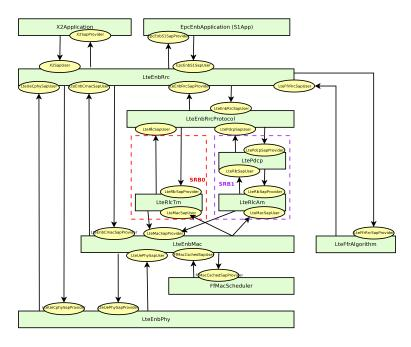
Figure 20.6: LTE radio protocol stack architecture for the eNB on the control plane
