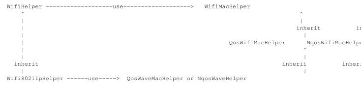
From the above diagram, Wifi80211Helper appears to be able to use any subclasses inheriting from Wifi-MacHelper; however, we force users to use subclasses only inheriting from QosWaveMacHelper or NqosWaveHelper. While the functions of WiFi 802.11p device can be achieved by WaveNetDevice's ContinuousAccess assignment, Wifi80211pHelper is recommended if there is no need for multiple channel operation. Usage is as follows:
