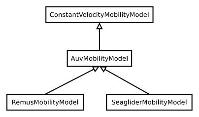
Figure 34.1: AUV's mobility model classes overview
