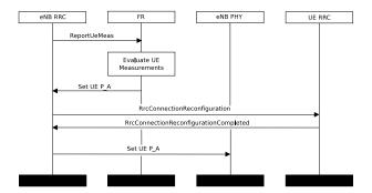
Figure 20.45: Sequence diagram of Downlink Power Control
