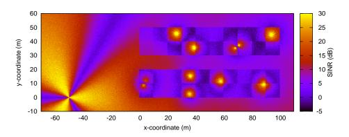
Figure 20.59: REM obtained from the lena-dual-stripe example
