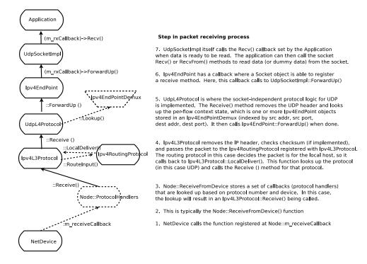
Figure 18.2: Receive path of a packet.
