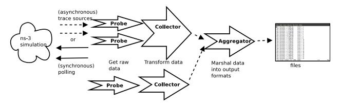
Figure 11.2: Data Collection Framework aggregation
