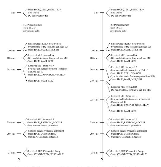
Figure 20.32: Sample runs of initial cell selection in UE and timing of related events
