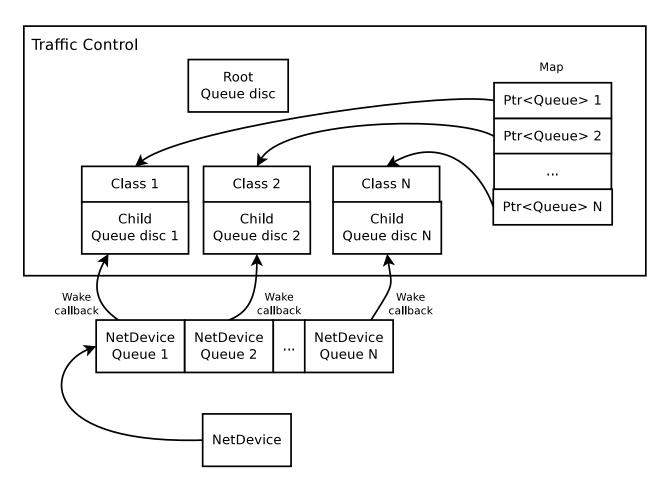
Figure 33.2: Setup of a multi-queue aware queue disc
