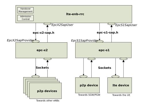
Figure 20.43: Implementation Model of X2 entity and SAPs
