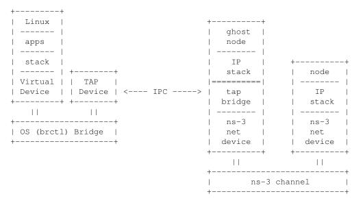
In this case, a computer running Linux applications, protocols, etc., is connected to a ns-3 simulated network in such a way as to make it appear to the Linux host that the TAP device is a real network device participating in the Linux bridge.
