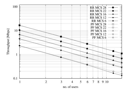
Figure 20.71: Test vectors for the RR and PF Scheduler in the downlink in a scenario where all UEs use the same MCS.
