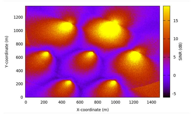
Figure 20.65: REM for RB 20 obtained from lena-dual-stripe simulation with Hard FR algorithm enabled
