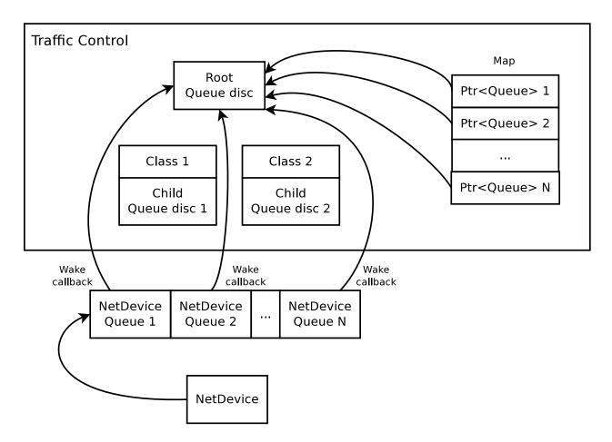
Figure 33.1: Setup of a queue disc (wake mode: WAKE\_ROOT)
