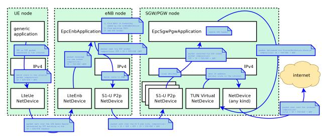
Figure 20.41: Data flow in the uplink between the UE and the internet
