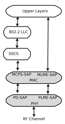
Figure 19.1: Architecture and scope of lr-wpan models
