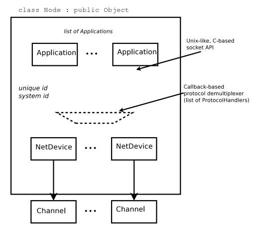
Figure 24.3: High-level node architecture
