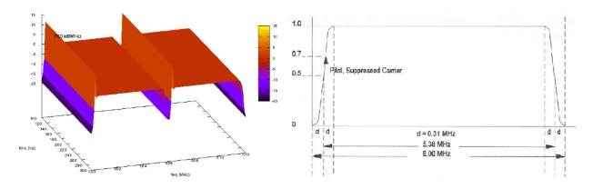
Figure 29.4: North America ATSC channel 19 & 20 signals generated using TvSpectrumTransmitterHelper (Left) and theoretical 8-VSB signal [Baron8VSB] (Right). Note that the theoretical signal is not shown in dB while the ns-3 generated signals are.
