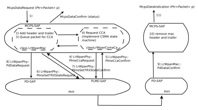
Figure 19.4: Data example for simple LR-WPAN data transfer end-to-end
