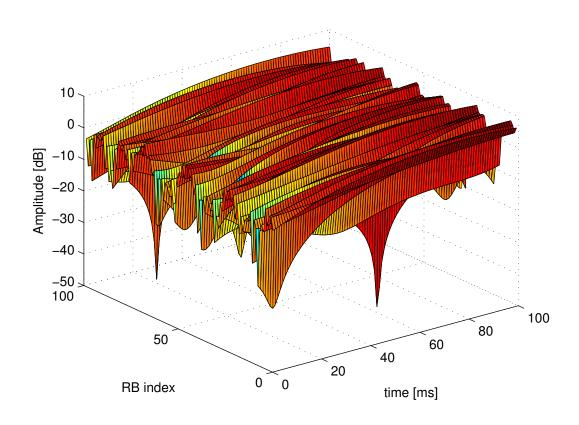
Figure 20.58: Excerpt of the fading trace included in the simulator for an urban scenario (speed of 3 kmph).
