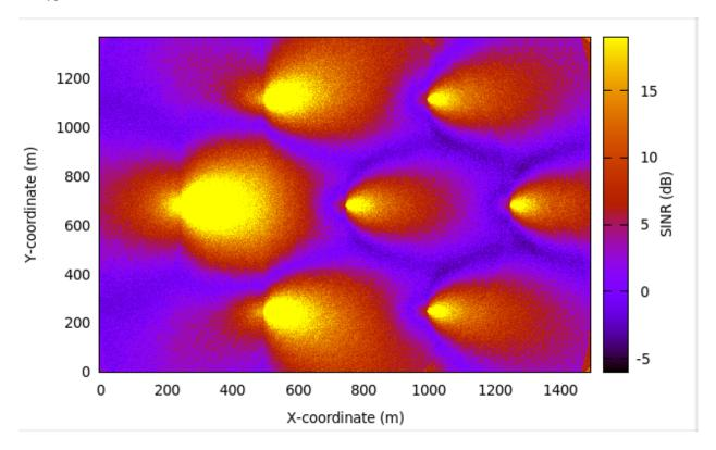
Figure 20.63: REM for RB 1 obtained from lena-dual-stripe simulation with Hard FR algorithm enabled
