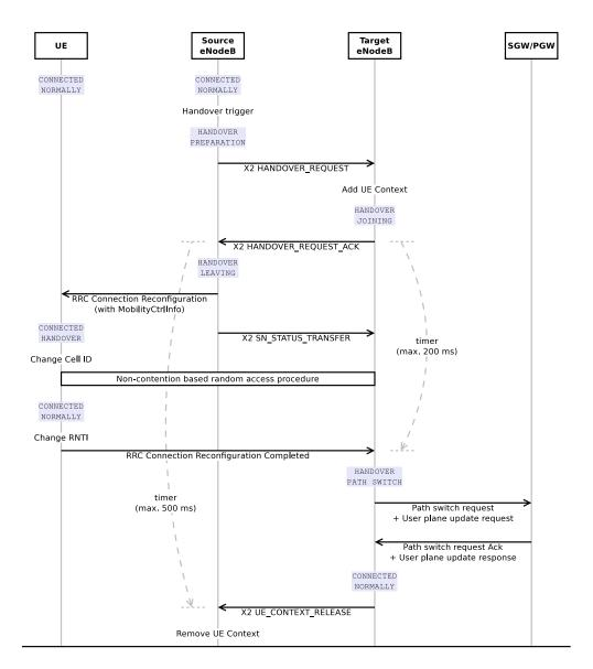
Figure 20.42: Sequence diagram of the X2-based handover
