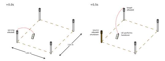
Figure 20.77: lte-handover-target test scenario in a 2×2 grid
