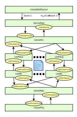
Figure 20.2: LTE radio protocol stack architecture for the UE on the data plane
