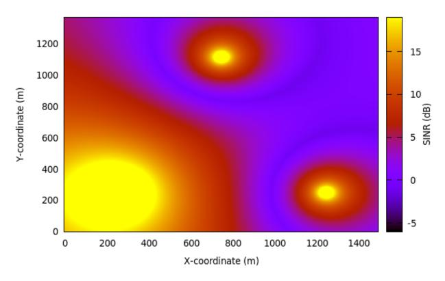
Figure 20.61: REM for RB 1 obtained from lena-frequency-reuse example with Soft FR algorithm enabled
