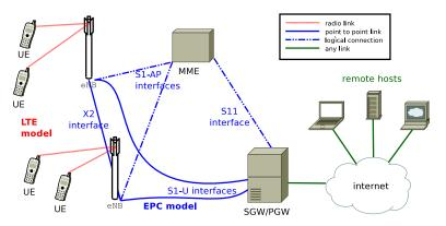
Figure 20.1: Overview of the LTE-EPC simulation model
