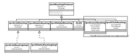
Figure 18.4: Ipv4Routing specialization.
