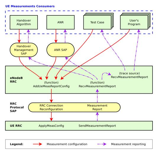
Figure 20.33: Relationship between UE measurements and its consumers
