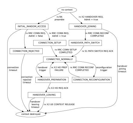
Figure 20.31: ENB RRC State Machine for each UE
