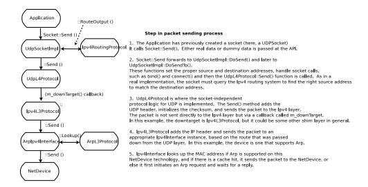
Figure 18.1: Send path of a packet.
