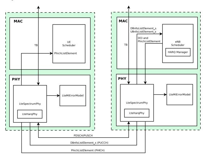
Figure 20.22: Interaction between HARQ and LTE protocol stack
