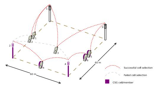
Figure 20.76: Sample result of cell selection test
