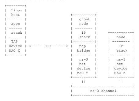
In this case, the pre-configured MAC address of the "Tap device" (MAC X) will not be the same as that of the bridged "ns-3 net device" (MAC Y) shown in the illustration above. In order to bridge to ns-3 net devices which do not support
