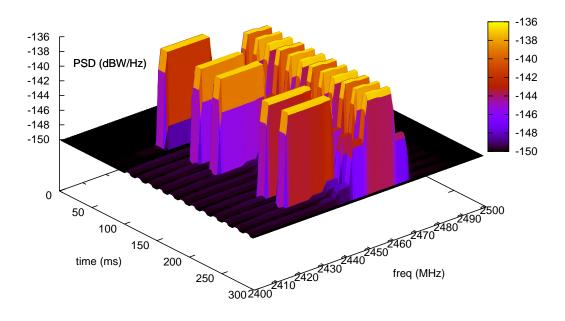
Figure 29.1: Spectrogram produced by a spectrum analyzer in a scenario involving wifi signals interfered by a microwave oven, as simulated by the example adhoc-aloha-ideal-phy-with-microwave-oven.
