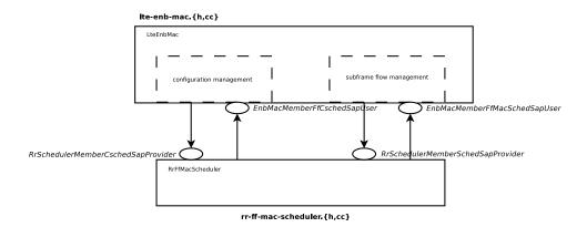
The same figure also shows, as an example, how the Round Robin Scheduler is implemented: to interact with the MAC of the eNB, the Round Robin scheduler implements the Provider side of the SCHED SAP and CSCHED SAP interfaces. A similar approach can be used to implement other schedulers as well. A description of each of the scheduler implementations that we provide as part of our LTE simulation module is provided in the following subsections.
