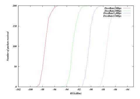
Figure 36.3: Clear channel (AWGN) error model for 802.11b
