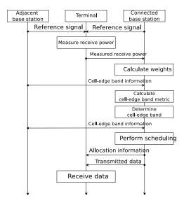
Figure 20.54: Sequence diagram of Distributed Frequency Reuse Scheme
