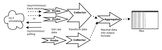
Figure 11.2: Data Collection Framework aggregation
